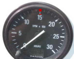
VACUUM PUMP TACHOMETER Should be run at NO LESS THAN 900RPM
